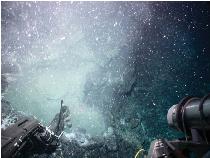
Fig. 2. The Alvin low-temp probe being inserted into a snow-blower located in a collapse structure at 10°44' N on the East Pacific Rise. Maximum temperatures reached only 9.5°C. Photo from forward-looking digital camera, Alvin dive 3937. Courtesy of J.R. Voight.
